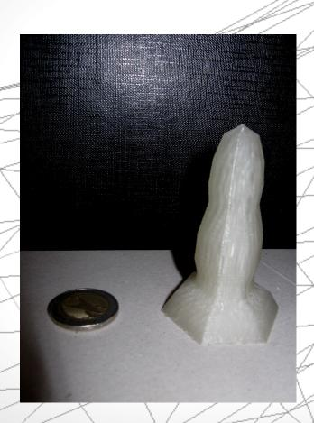
The first printing test was a simple revolution solid with 6\*10 mesh points (very pointy)
